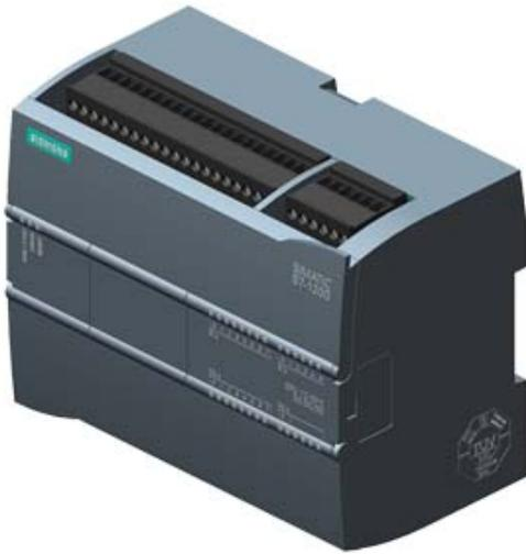
SIMATIC S7-1200F, CPU 1215 FC, KOMPAKT CPU, DC/DC/DC, 2 PROFINET PORT, ONBOARD I/O: 14 DI 24VDC; 10 DO 24VDC; 0,5A; 2 AI 0-10V DC, 2 AO 0-20MA DC, STROMVERSORGUNG: DC 20,4 -28,8 V DC, PROGRAMM/DATENSPEICHER 150 KB
