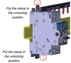
Pull the device forward in order to release it from the rail
