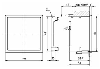
Picture 7: Dimensional drawing FQ0107, FQ0207, FQ0307 in FQ0407 (all dimensions are in mm)
