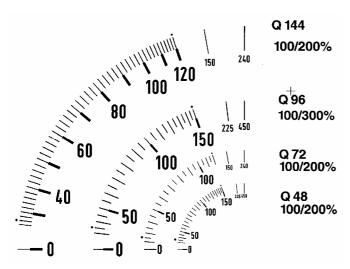
Picture 3: Drawing of scale: Version with overload (ammeters)
