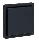
This surface-mounting intermediate switch is equipped with with plug-in terminals and is to be mounted in a splashproof, surface-mounting box. The entire unit is splashproof which makes it extremely well-suited for use in damp areas and in demanding environments. Colour combination: black. The Niko Hydro products are not suitable for use in ammonia rich environments (e.g. pig houses).
