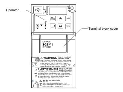
Open the terminal block cover to wire the main circuit terminal block and the control circuit terminal block.
