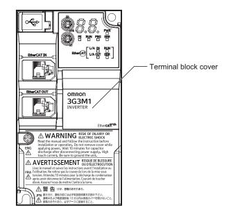
Open the terminal block cover to wire the main circuit terminal block and the control circuit terminal block.
